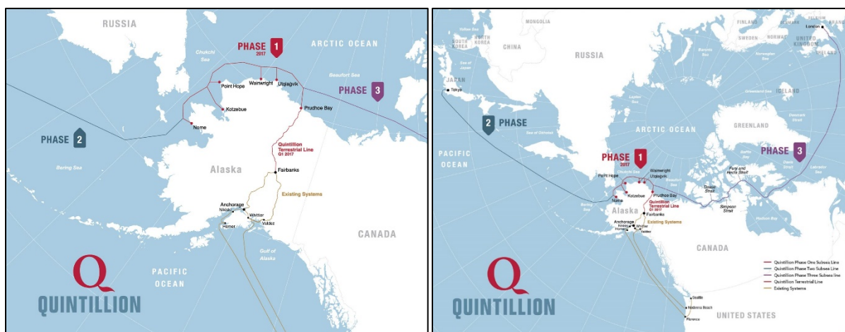
Figure 6-20 The three phases of the Quintillion Subsea Cable System. Phase 1 was completed in 2017
